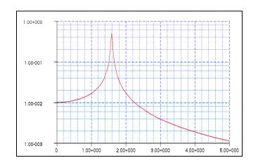
Transient analysis with a unit force applied to the spring at 1.59 Hz
